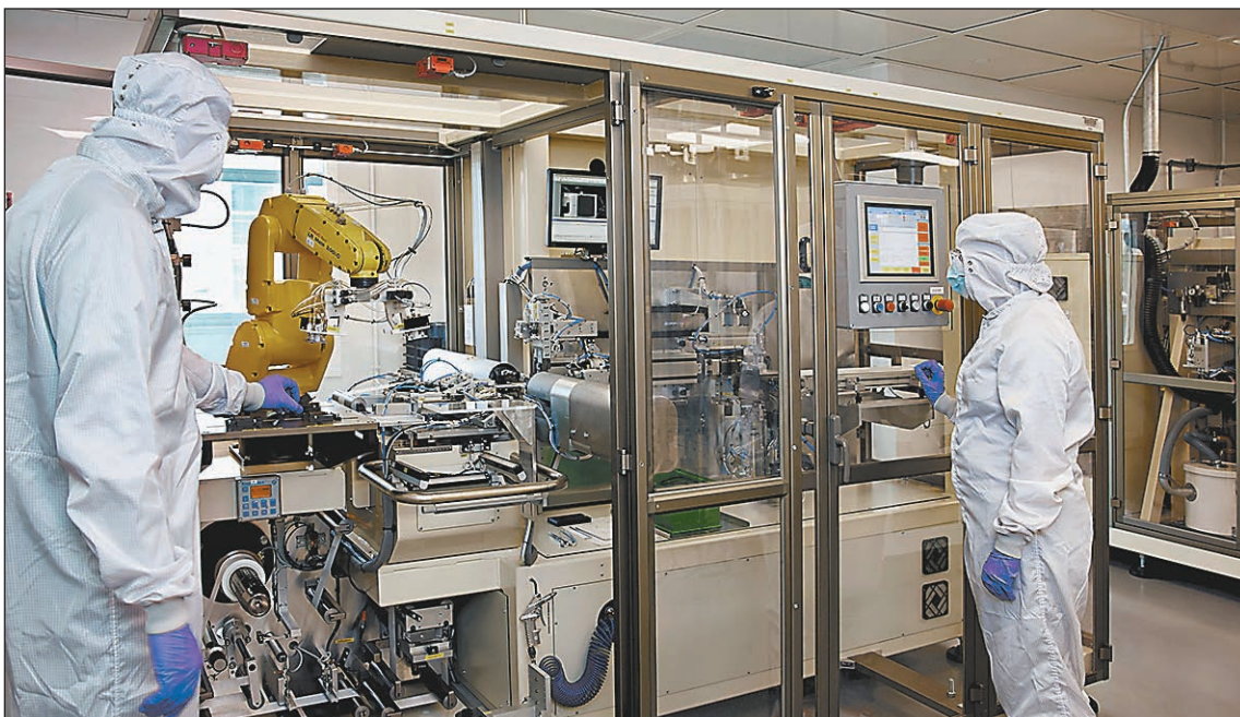
GM battery Research and Development electrochemists build prototype battery cells using a robotic battery cell stacking machine. Work done on batteries over the past decade at GM R&D will be moved forward at the new Wallace Battery Cell.
