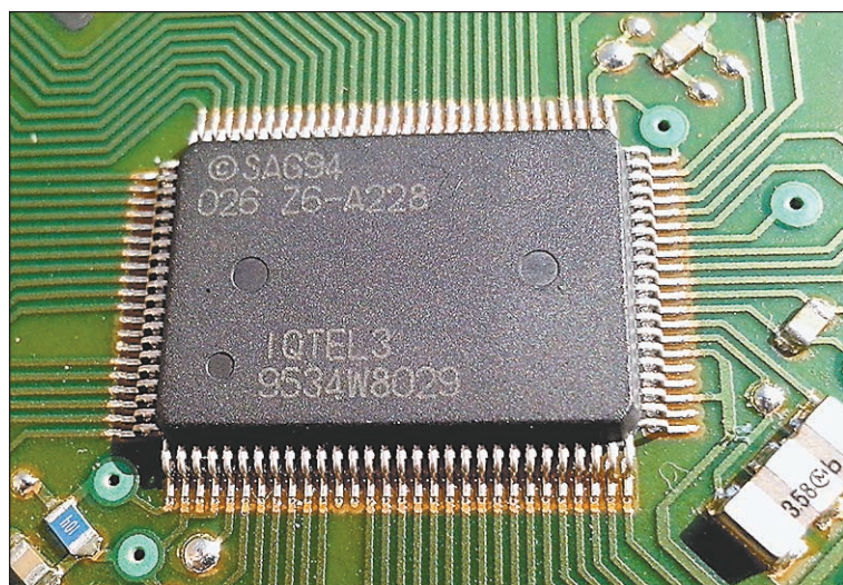
A typical computer chip used in vehicles (magnified). courtesy of GM
