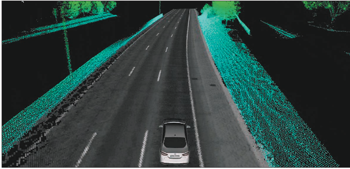
Ford is gathering LIDAR data as part of the company's efforts to develop a working AI vehicle for the future.
