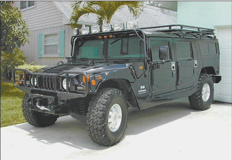
This 2006 Hummer H1 Alpha Wagon came equipped with a GM Duramax diesel engine and weighed 7,847 pounds and averaged about 15 miles to the gallon.
