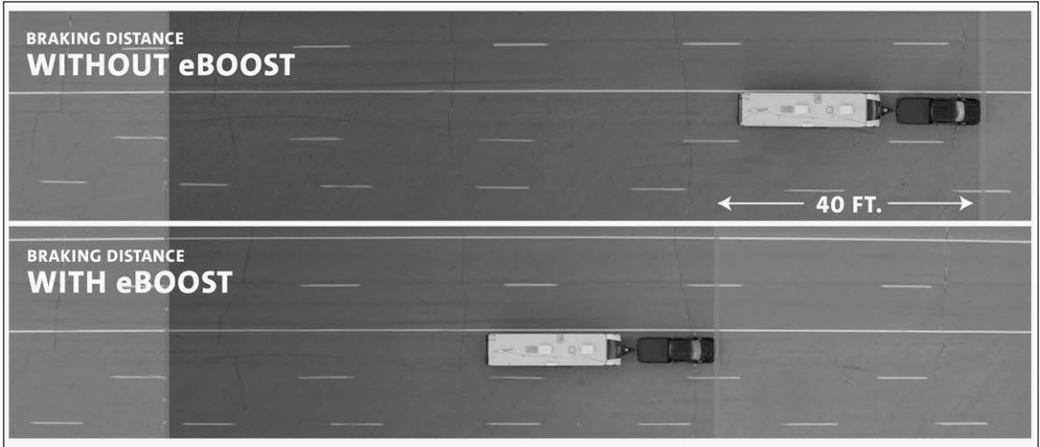
This shows how GM's advanced concept brake system shortens stopping distances of trucks towing big loads.
