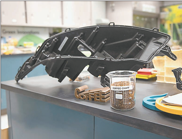
Ford and McDonald's are using coffee bits to make automotive parts.
