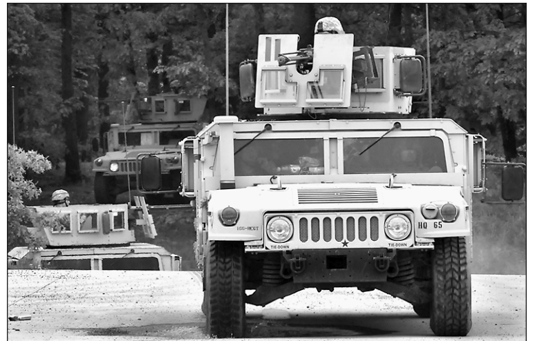
System in this armored HMMWV gun-truck aids in preventing rollovers.
