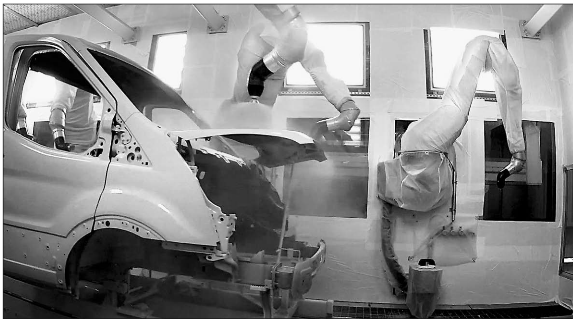
Paint applied through the new process will retain 90 percent of its gloss at four years in service.
