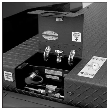
The CNG "on" switch
