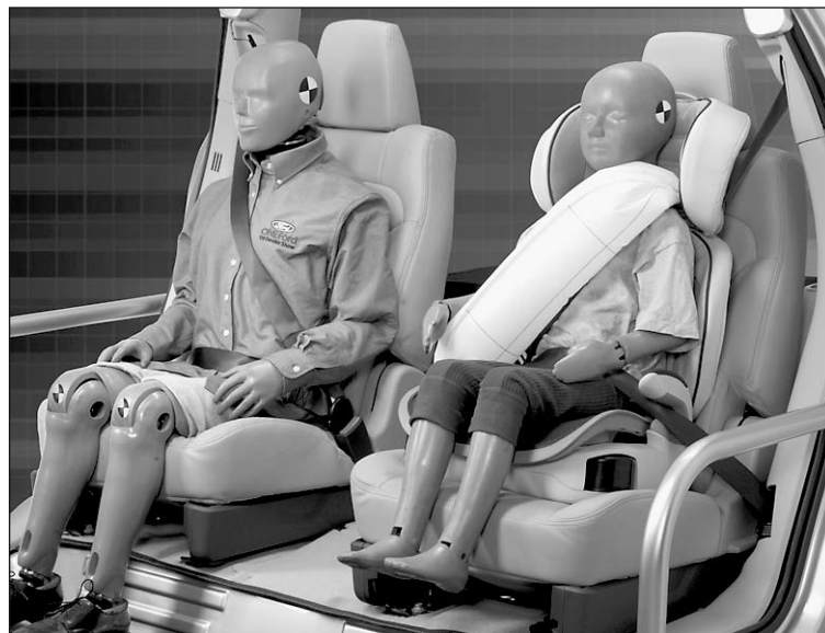
Ford's first-ever production inflatable seat belts are designed to help reduce head, neck and chest injuries for rear-seat passengers.
