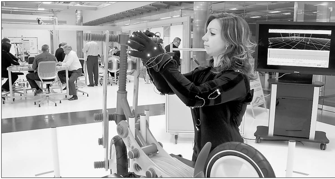
A WCM Academy student wears a motion capture suit to show movements required to build a child's bike.
