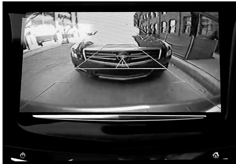
A set of colored guidelines appear on the center stack display when in reverse, to mark the vehicle's turn radius and allow for easier parking and backing maneuvers.
