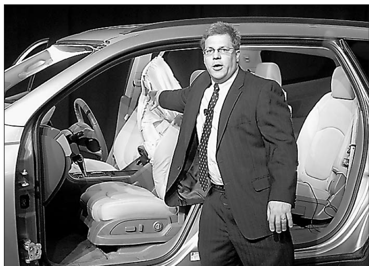
General Motors Advanced Restraint Systems Senior Staff Engineer Scott Thomas demonstrates the industry's first front center air bag in the fall of 2011 at the GM Proving Ground.
