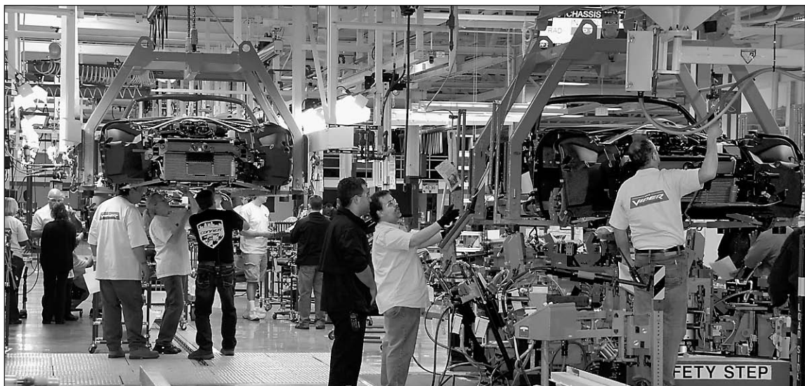
Employees at Chrysler's Conner Avenue Assembly Plant work on the chassis of the next generation SRT Viper. On the right, the rolling chassis is placed on the aligner to ensure proper camber alignment. Nearly 150 employees hand build 12 of the legendary American muscle cars each day.
