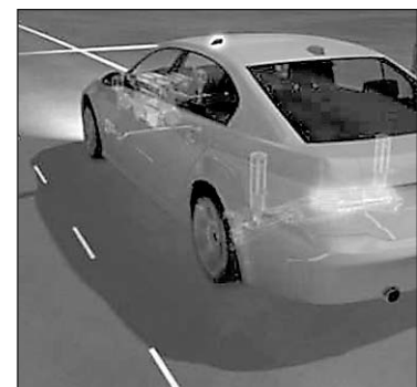
Lane keeping assist tracks lane markings and puts torque on the steering wheel to guide the car back to the center if it strays.
