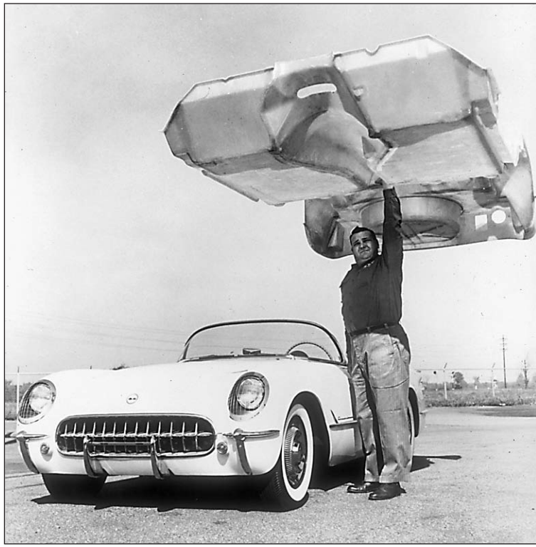
1953 Corvette featured a lightweight fiberglass body.
