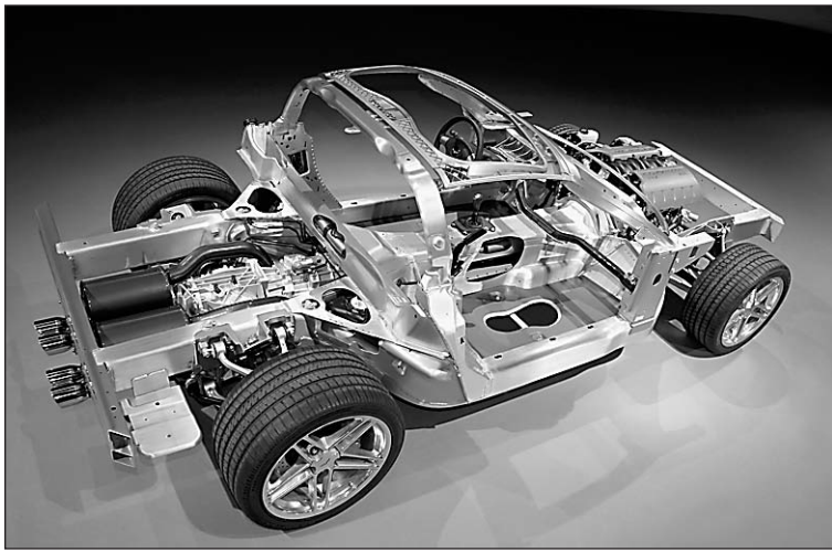
The 2006 Corvette Z06 introduced a unique aluminum-intensive chassis.
