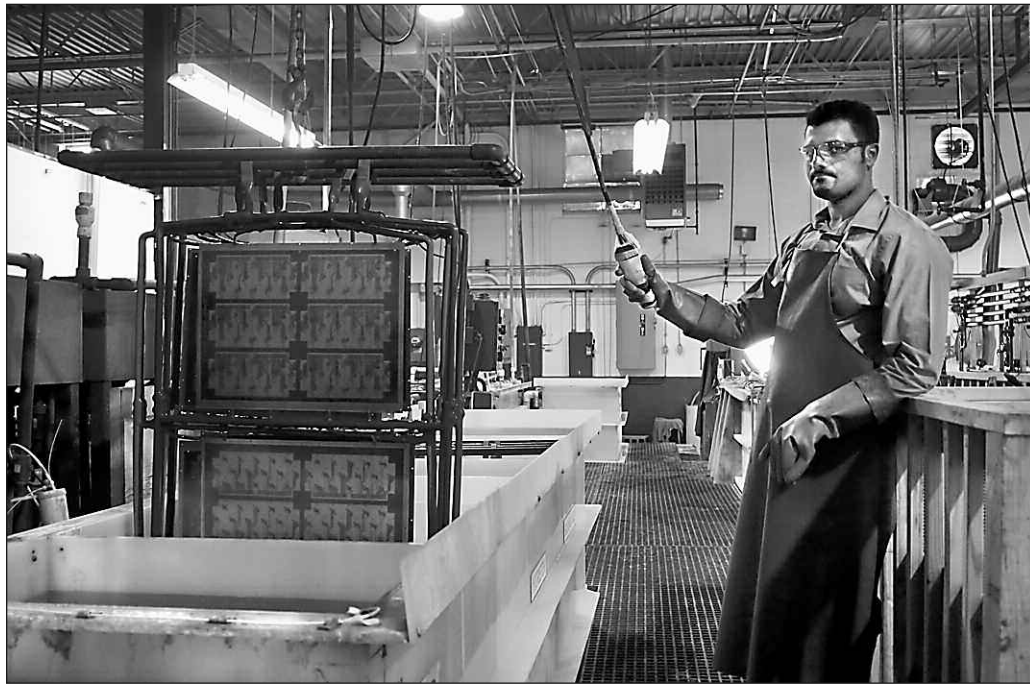
Circuit boards undergo cleansing baths at K & F Electronics.
