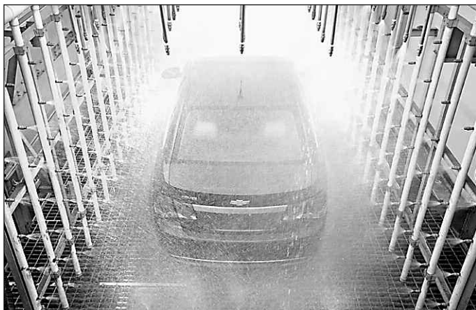
The 2012 Chevrolet Cruze blasts through thousands of gallons of water while undergoing hi-tech weather testing in the Universal Water Test Booth at the General Motors Milford Proving Ground in Milford. Using 330 nozzles, 825 gallons of water are sprayed onto the car each minute. The intensity of the test exposes weaknesses in the car's seals, which experts can resolve to help ensure drivers and passengers stay dry in a rainstorm.
