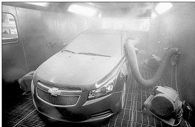
The 2012 Chevrolet Cruze undergoes hi-tech weather testing in the Dust Booth at the General Motors Proving Ground in Milford. The Dust Booth exposes the car to an extreme number of dust particles to help keep it airtight. The number of auto test labs that run a GM car through various trials before it is released to the customer has increased over the years, all to help GM engineers know that they are ensuring the highest quality standards.
