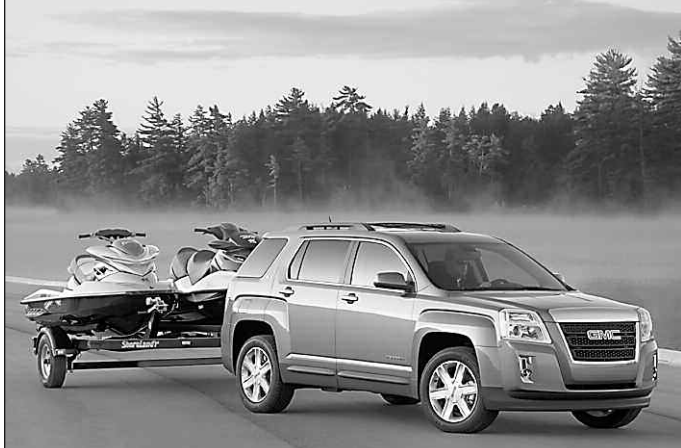
Standard StabiliTrak stability control, with Trailer Sway Control, is standard on all GMC vehicles, including the Terrain Small SUV, which can tow up to a class-leading 3,500 pounds. Sway control uses sensors to measure the yaw created by unexpected side-to-side motions created by a trailer. The vehicle automatically corrects those motions by applying individual brakes to bring the vehicle and trailer back in line.
