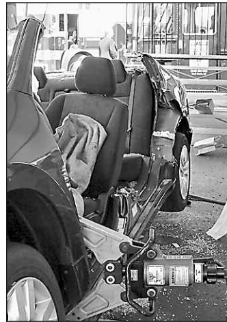
Note the jaws of life, foreground, from the Livonia Fire Dept., which did a demo of how their firemen cut open this Nissan Sentra, built with a high-strength steel interior.
