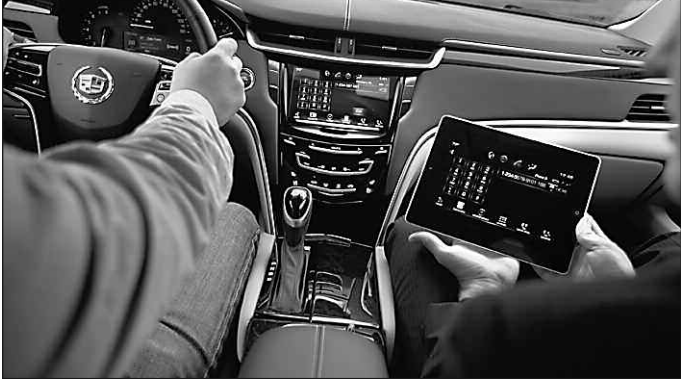
A Cadillac CUE App that enables shoppers to "test-drive" the system on an iPad, anytime, anywhere. The CUE app replicates many of the controls and features of the CUE center stack. The CUE center screen and control panel represents the first automotive use of capacitive touch and familiar multi-touch gestures. Every 2013 Cadillac XTS sold in the U.S. includes an iPad customized just for Cadillac buyers.
