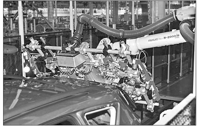
Auto plant assembly work previously performed by UAW employees including the installation of the instrument panel, windshield, roof and fenders, are now all being performed by robots equipped with cameras and laser eyesights.
