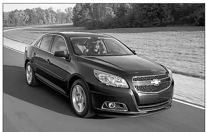
Chevrolet says that the Eco version of the Malibu, above, with electric steering, improves fuel economy by up to 2.5 percent over conventional, hydraulically steered cars.
