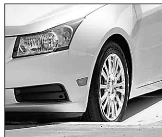
Chevrolet Cruze drives through the pothole course at the General Motors Proving Ground in Milford, Mich. The potholes are engineered to simulate severity of road damage and recreate varied load conditions that occur in a vehicle when it is driven through one.
