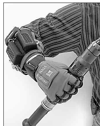
The Human Grasp Assist, based on the robotic hand of General Motors' and NASA's Robonaut 2, is designed to allow the wearer to hold a grip longer and more comfortably. The glove, still in prototype stage, is expected to be used in space and applied to manufacturing plant use on Earth.
