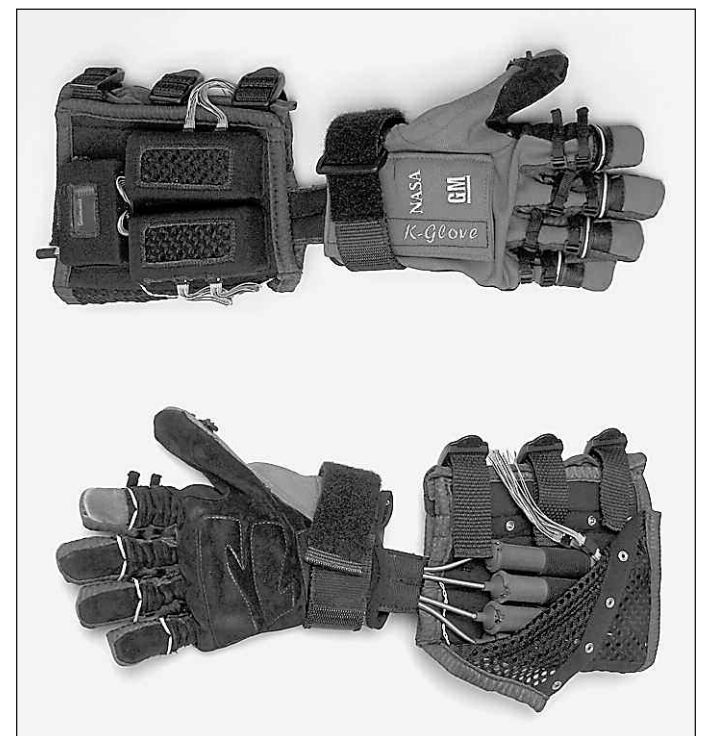
The Robo-Glove (officially known as the Human Grasp Assist) when fully developed, is expected to reduce auto workers' risk of repetitive stress injury. The glove uses leading-edge sensors, actuators and tendons comparable to the nerves, muscles and tendons in a human hand.
