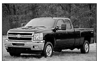
The 2013 bi-fuel Chevrolet Silverado HD includes a compressed natural gas (CNG) capable engine that seamlessly transitions between CNG and gasoline fuel systems. Combined, the truck offers a range of more than 650 miles.
