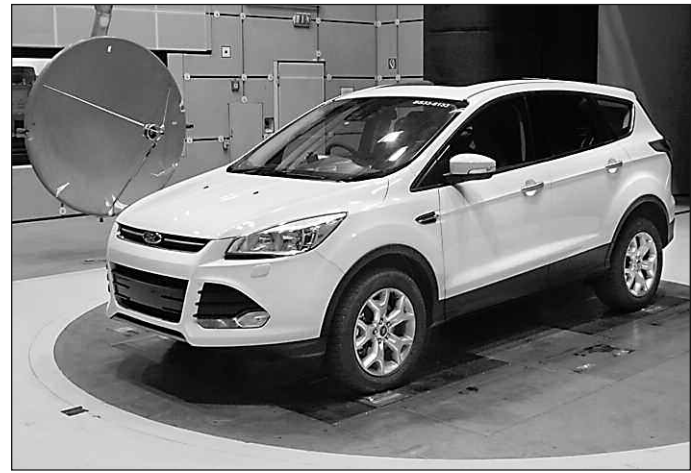
Ford's elliptical mirror helped make the all-new Ford Escape the quietest Escape ever.
