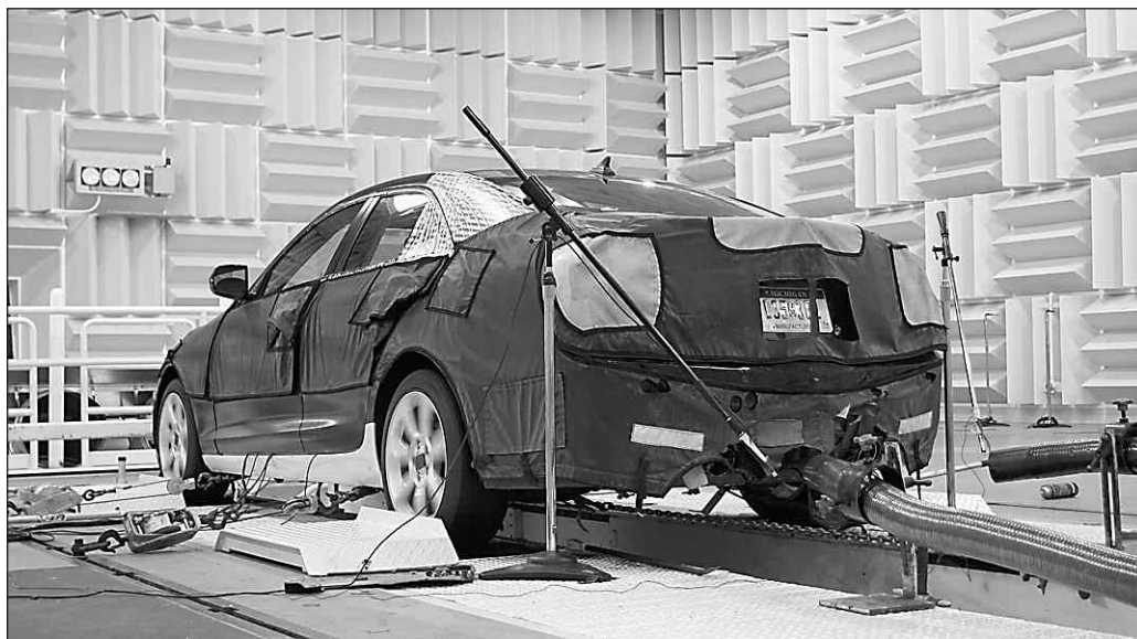
The 2013 Cadillac ATS undergoes careful sound testing in labs at GM's Milford Proving Ground.
