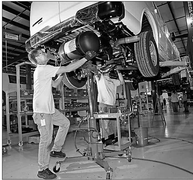
Darren Weatherly, left, and Robert Williams install CNG tanks on a Chevrolet Express cargo van being outfitted to operate on compressed natural gas at the IMPCO plant in Union City, Ind. CNG-powered vans can produce approximately 25 percent fewer emissions than similar gasoline and diesel-powered vans.
