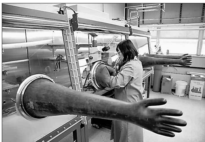
Meng Jiang, a GM researcher in Warren, prepares to look at lithium-ion battery components through a microscope that is housed in an argon gas-filled "glove box." The lithium-ion battery components are sensitive to oxygen and humidity.
