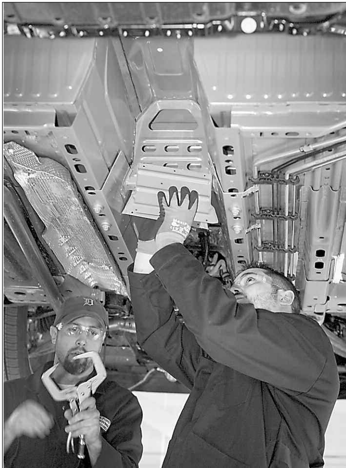
General Motors engineers fit structural modifications to further protect the battery pack of the Chevrolet Volt. The structural enhancements will more evenly distribute crash energy, GM says.
