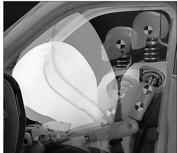
TRW's dual contour passenger airbag is capable of adjusting both the airbag pressure and size to help tailor protection according to occupant size and other variables of a crash.
