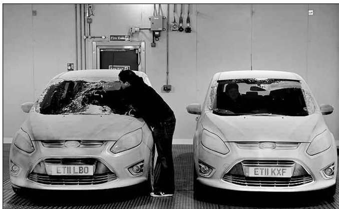
Ford Quickclear technology helps to clear windshields of ice at the click of a switch (right), which is more comfortable than scraping (left).
