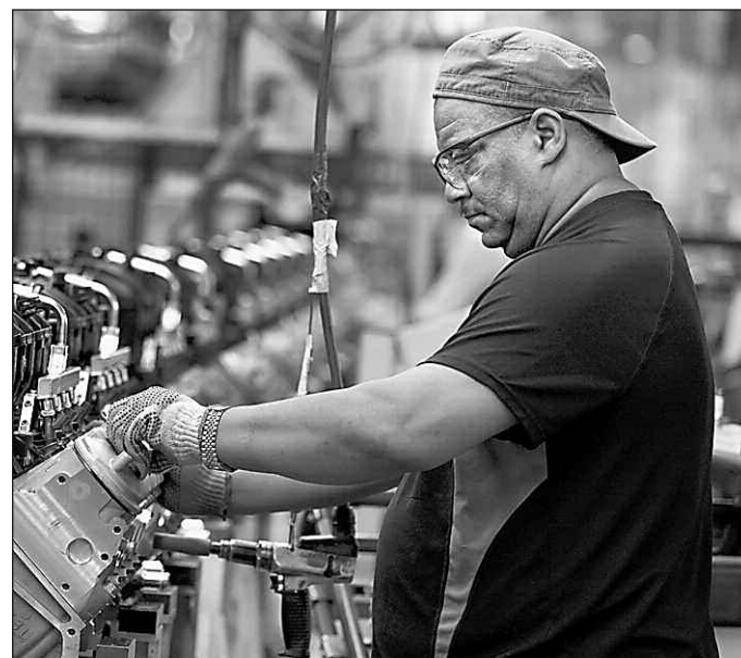
General Motors Romulus Engine Plant employee Winfred Pride installs a rocker cover on an 8-cylinder engine.
