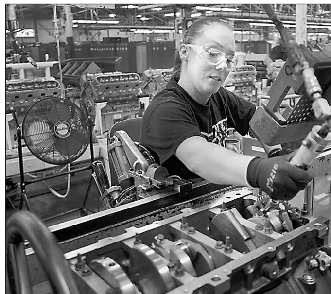
GM Romulus Engine Plant employee Christy Seay stuffs a piston into an 8-cylinder engine. General Motors announced last week it will invest $385 million to prepare the facility for production of an all-new, fuel-efficient engine program.
