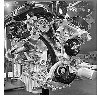
The 3.7L V6 Ford engine powers the 2011 F-150 4 x 2 Supercrew.
