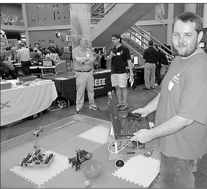
LTU sophomore Jon Nabozny with his entry at Lawrence Tech's first-ever Robo Expo. Nabozny's robot uses an IBM Thinkpad's mounted web-cam for guidance, together with batteries, wheels and a motor for locomotion on his ground robot.
