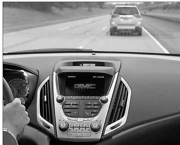
The 2012 Terrain exclusively uses a single camera mounted in the windshield to help avoid front-end and lane departure crashes.
