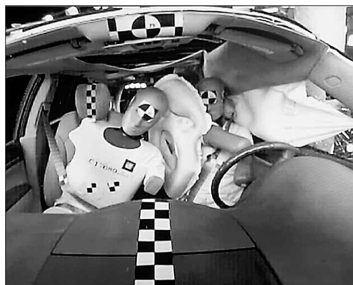
Crash test dummies involved in a side impact collision demonstrate GM's new front center air bag.
