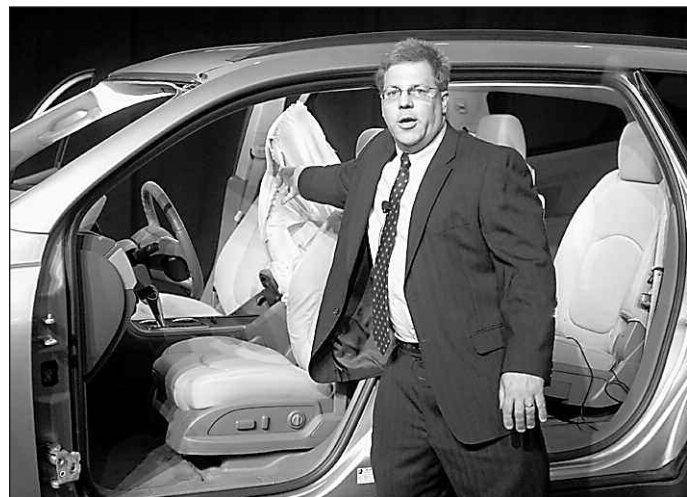
General Motors Advanced Restraint Systems Senior Staff Engineer Scott Thomas demonstrates the industry's first front center air bag, an inflatable restraint designed to help protect drivers and front passengers in side impact crashes.
