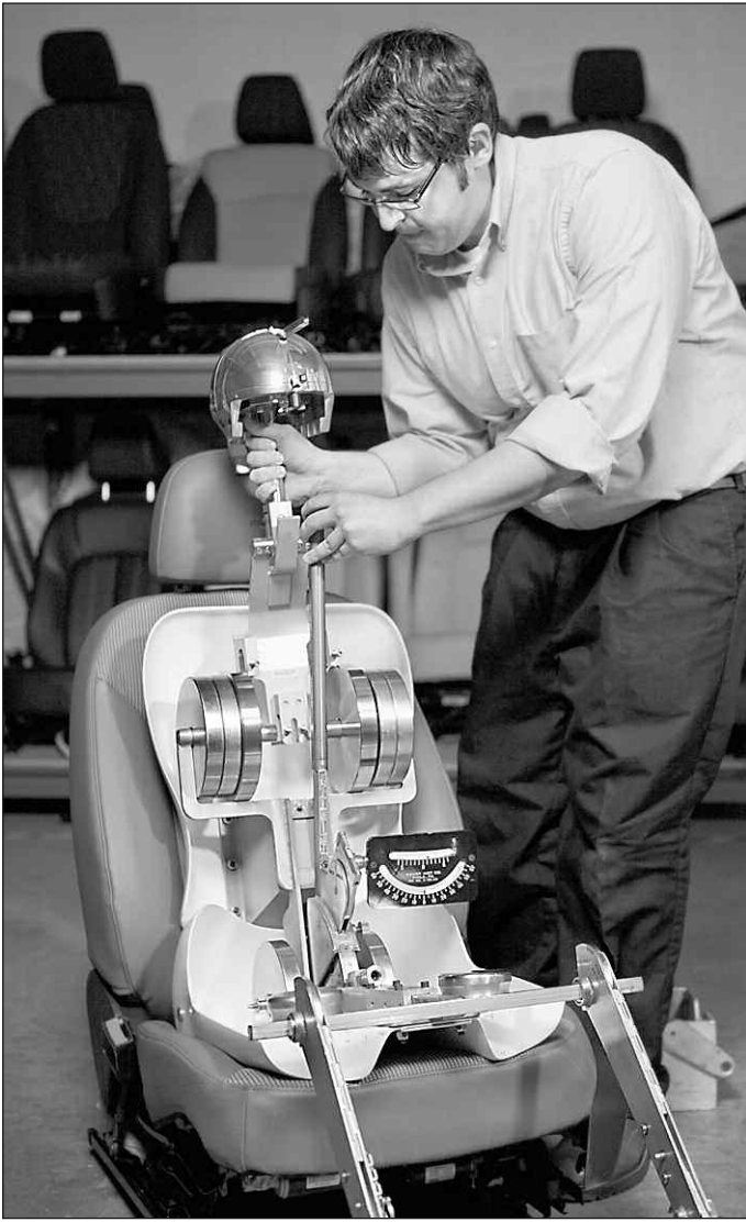
Chevrolet Malibu Seat Performance Engineer Daniel Cohen adjusts Oscar, General Motors' mannequin-like simulation tool used early in the product development process to provide key vehicle interior measurements at the General Motors Milford Proving Ground. The data generated by Oscar helps engineers and designers to create optimal interior space and comfort for vehicles like the new 2013 Malibu.
