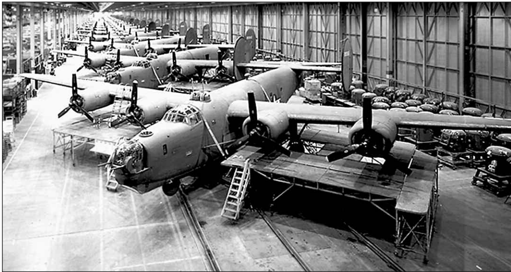
The Ford Willow Run Bomber Plant's B-24 Liberator assembly line during World War II.
