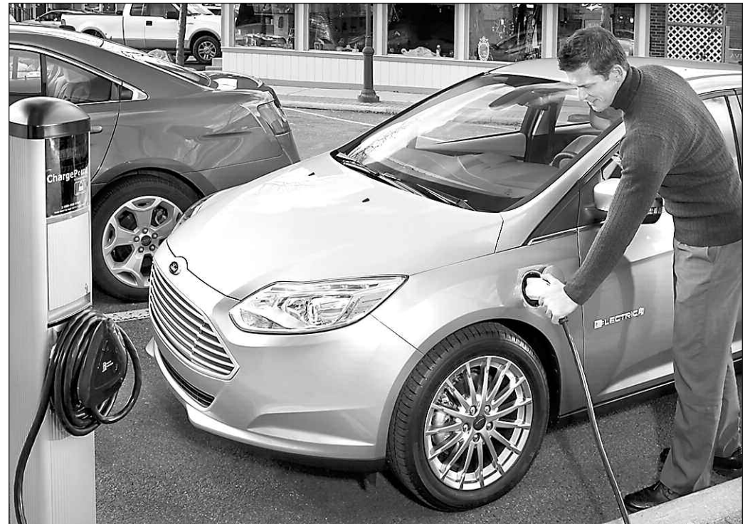
Ford engineers researched several locations for the Focus Electric and C-MAX Energi charge ports to ensure the port was in the best possible place for customer use.
