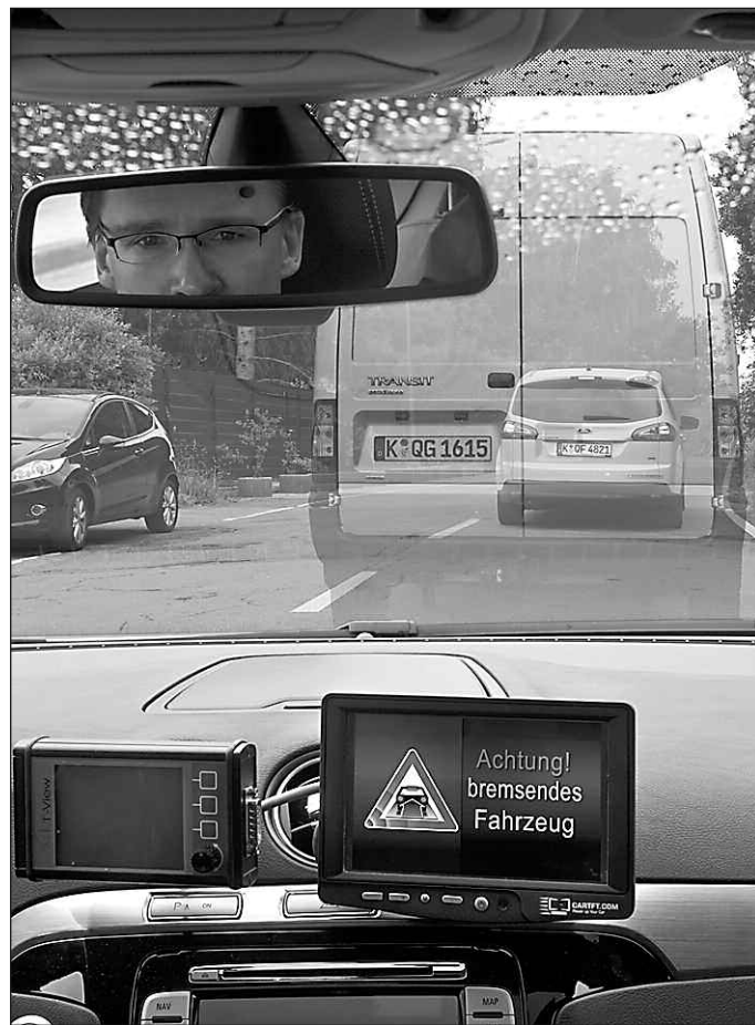
Two S-MAX vehicles demonstrated Ford's developmental vehicle-to-vehicle warning system – for example, hard braking of the lead S-MAX triggers an emergency signal that is displayed inside.
