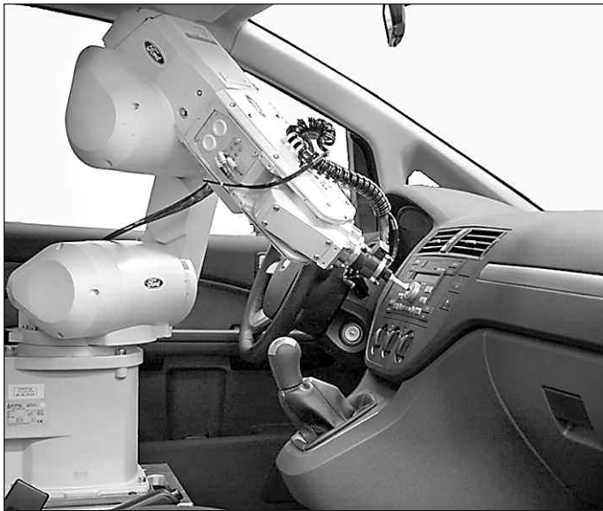
Ford uses an interior robot named Ruth at its plant in Germany.
