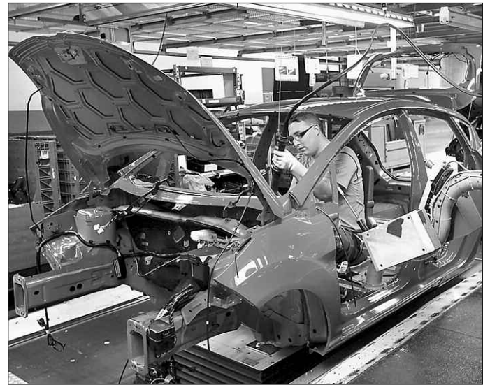
Ford's new "happy seat" allows assembly line workers to sit and swivel into tight workspaces as the chassis moves down the line.
