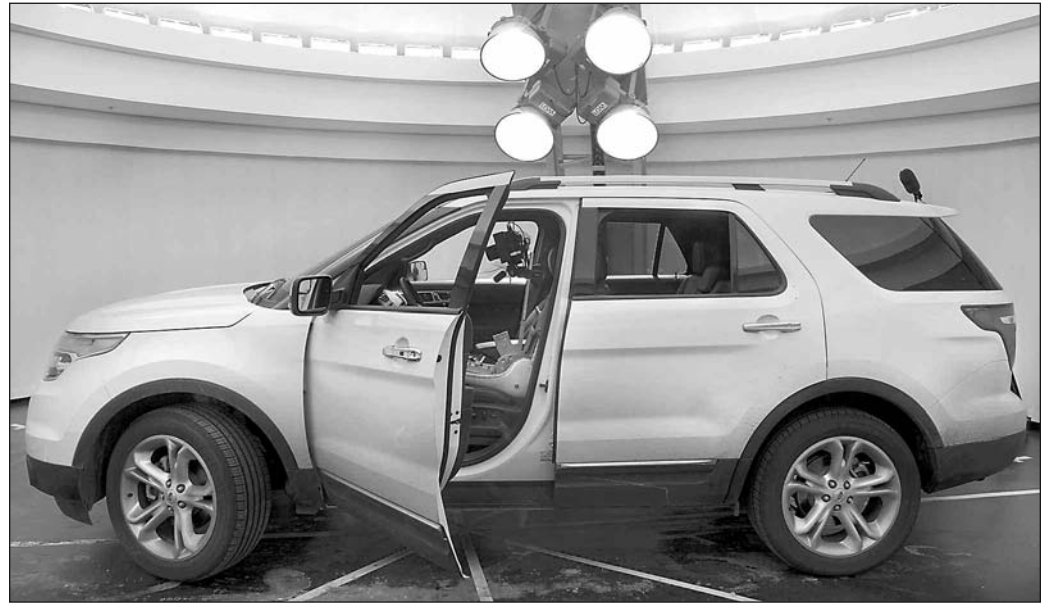
Ford's Visual Performance Evaluation Lab puts the proverbial spotlight on lighting and glare issues that customers may face, as it mimics sunlight conditions from dawn to dusk.
