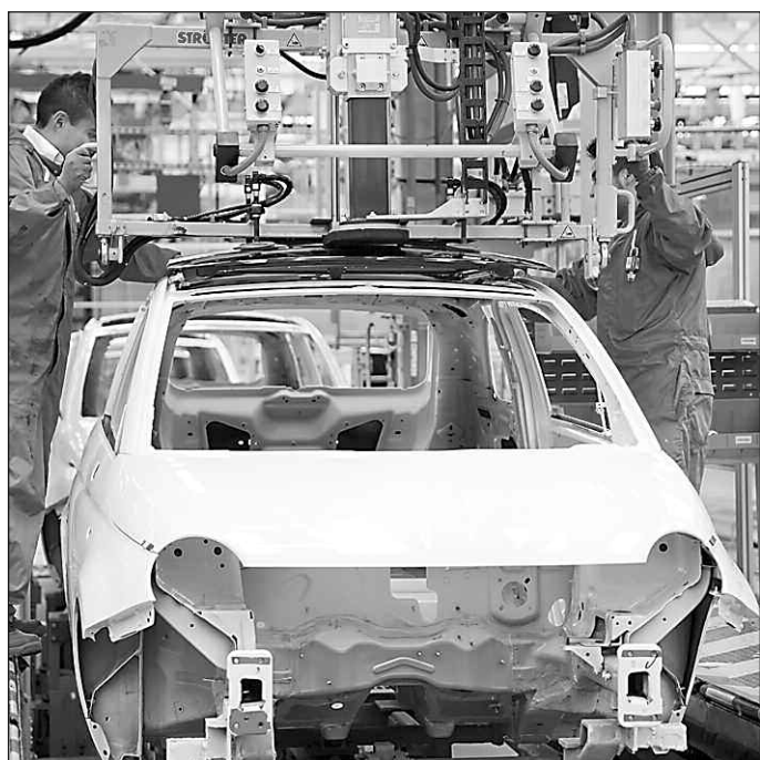
Employees at Chrysler Group LLC's Toluca (Mexico) Assembly Plant install the sunroof on the all-new Fiat 500. The Toluca facility has been building various Chrysler vehicles for domestic and export markets for more than 40 years. The plant began producing the Fiat 500 in December 2010.
