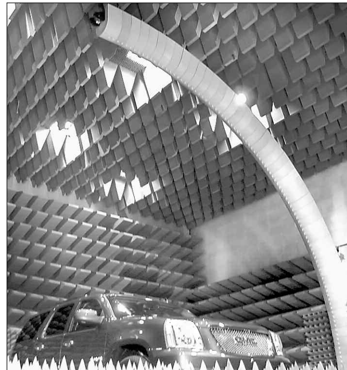
A 2011 GMC Yukon Denali undergoes antenna reception testing by General Motors' SATIMO Arch at the GM Proving Ground in Milford. The Antenna Testing System beams signals from 103 discrete probes down to a vehicle on a rotating platform to determine optimum antenna placement.
