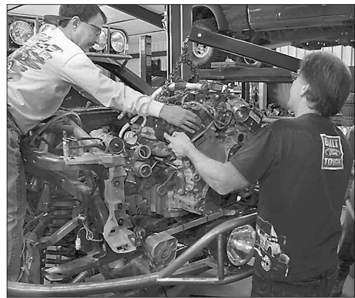
Ford engineers will disassemble and examine the 3.5-liter EcoBoost "hero" truck engine for long-term durability in front of the public at the North American International Auto Show in Detroit on Jan. 15.
