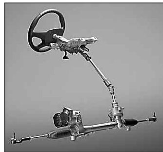
Belt drive steering is being added to the Ford Focus platform in Europe.
