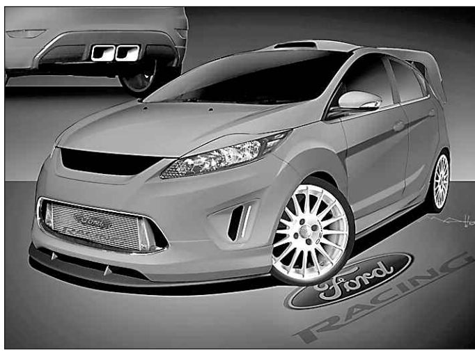
Ford Fiestas will take center stage this year Specialty Equipment Marketing Association. Pictured is a Ford Racing Fiesta Concept with a 2.3-liter EcoBoost engine capable of 350 horsepower.
